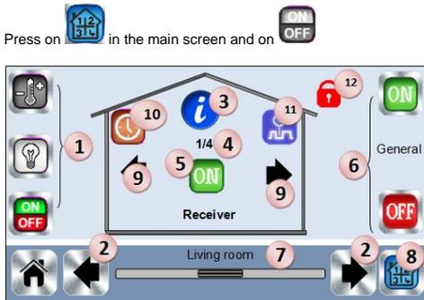
1. Device type choice (heating, lighting, On/Off). These buttons are only displayed if one device type is installed in the room (colored if active).
